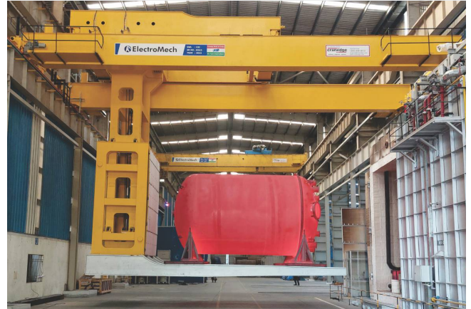
Furnace Loading Crane
