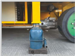
Jacking Provision For effortless and quick replacement of tyres.
