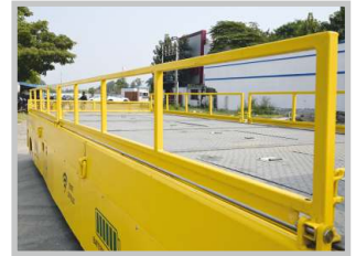
Side Guards (Optional) Avoid accidental load slippage.
