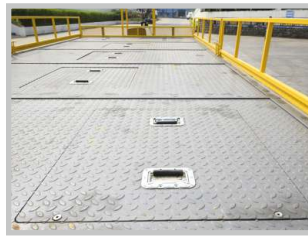
Removable Cover Easy access to battery and motor components during maintenance.
