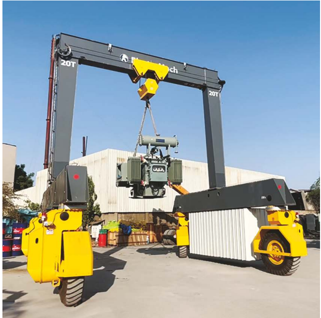
Handling of large transformers in a storage yard
