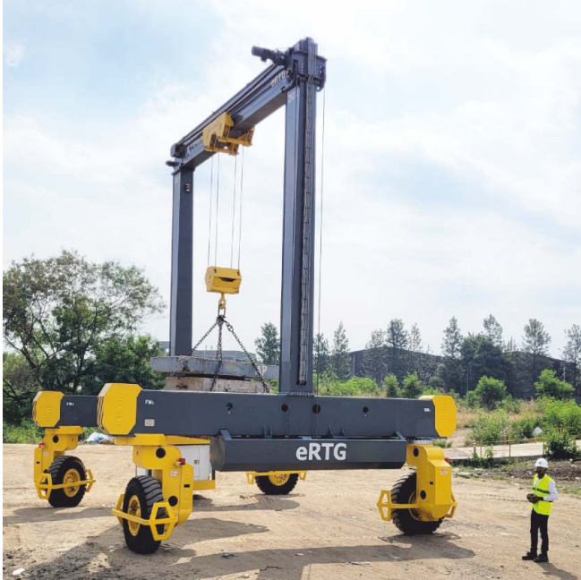
Pivoting motion using 2-wheel steering with 20t load
