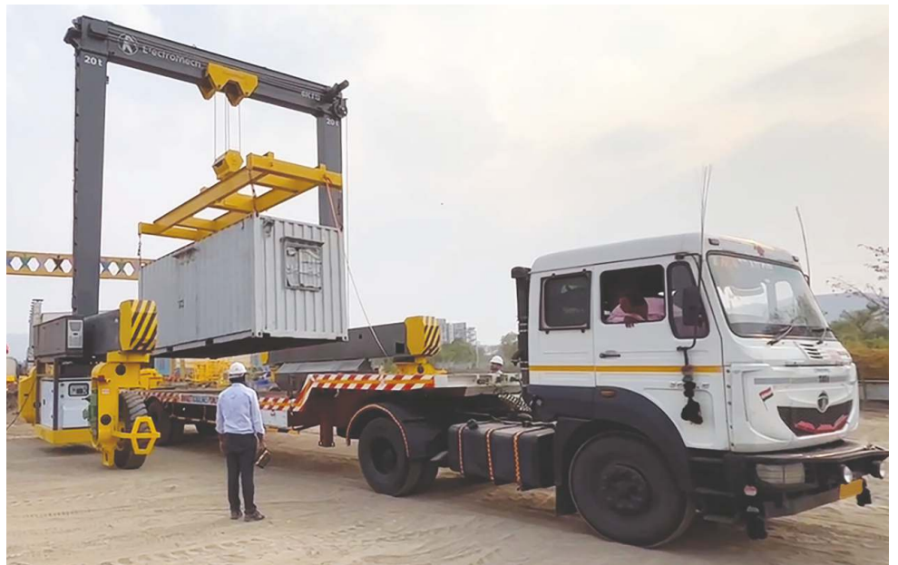
Handling of 20 feet shipping container
