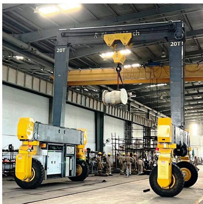
Valve parts handling (indoor application)
