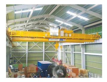
ElectroMech manufactures Double Girder Overhead Cranes in SWLs ranging from 1000kg to more than 300t.
