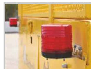
Flashing Light with Built-in Hooter Audio-visual alarm while the STC is moving
