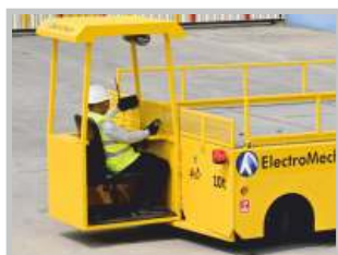
Operator's Cabin (Optional) Useful for outdoor operations and areas requiring long travelling distance
