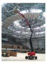
Working Height 15.7m to 26.6m Load Bearing 227kg to 250kg Gradeability 30%, 40%, 45%
