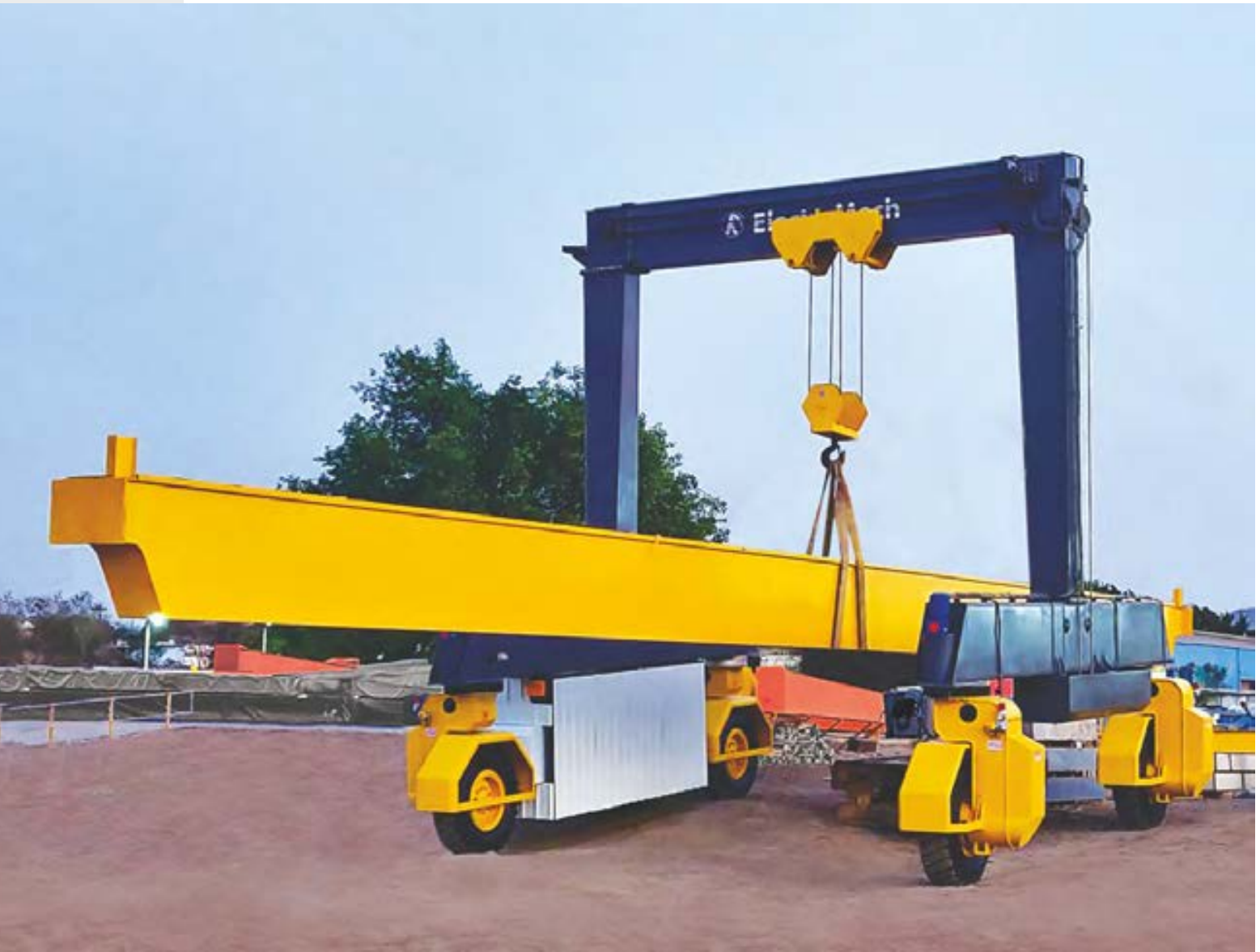
eRTG - Rubber Tyred Gantry crane for handling fabricated girder
