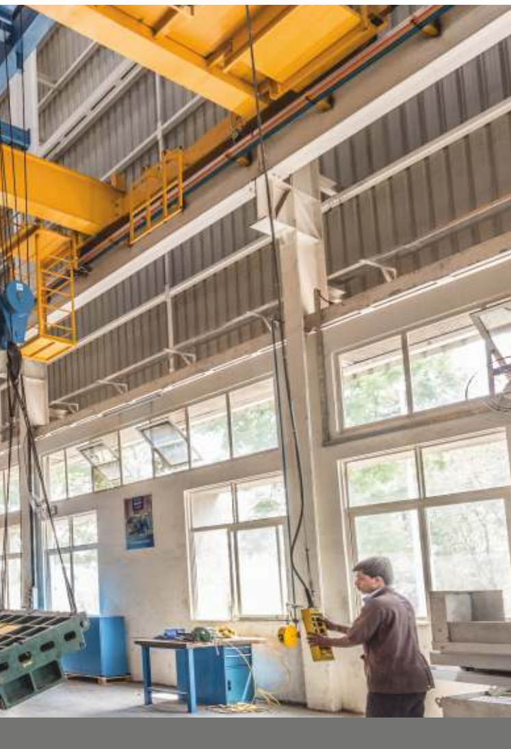
20/10MT, 8.8m span semi-gantry and 35/10MT, 21.3m span double girder cranes at Bajaj Auto Ltd. for handling and tilting of dies
