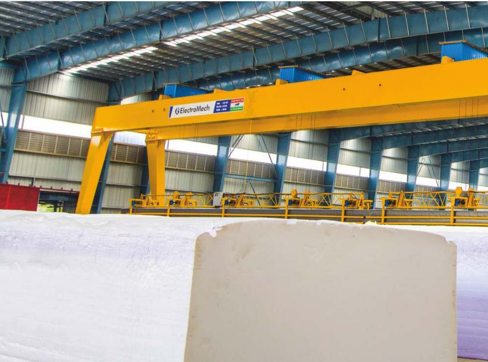
Double girder gantry crane with 54.6m span for handling and stacking of 52m long foam blocks
